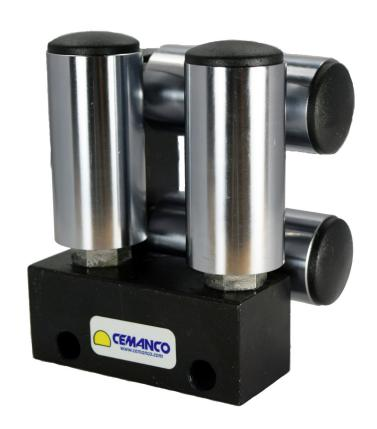
Non Adjustable Roller Cross with 4 - 30 x 60mm Steel Polished Rollers Hardened (62 +/- 2 HRC) (High Quality Bearing) for a Max 20mm Material
